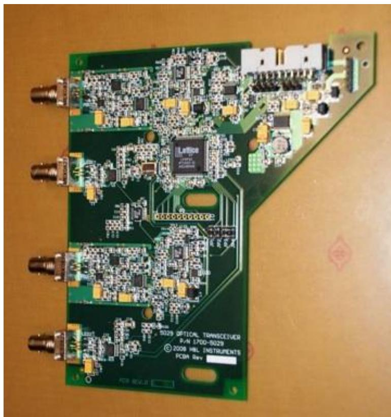
The board above works just fine after the treatment and, thanks to the nickel surfaces, will continue to work reliably without the doubt of a tin whisker induced failure. So far, not one assembly to which the process has been applied has failed to function after the process exactly as it did before.
